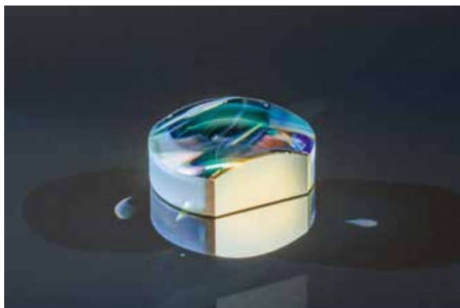
Figure 16: Solderable coating on the side of a lens
