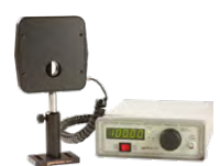
SDC-500 digital optical chopper
