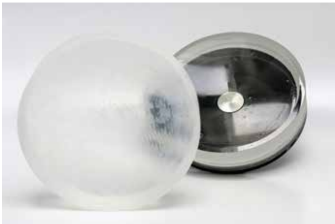
Figure 11: Parabolic substrate in production process, before (l.) and after lapping and polishing (r.)
