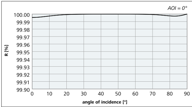
Figure 3: Reflectance vs. AOI of a wide angle scanning mirror for polarized Nd:YAG laser radiation: HRs (0° – 90°, 1064 nm) > 99.9 %
