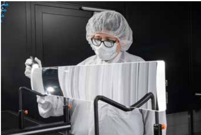
Figure 18: Quality control of large scale optics
