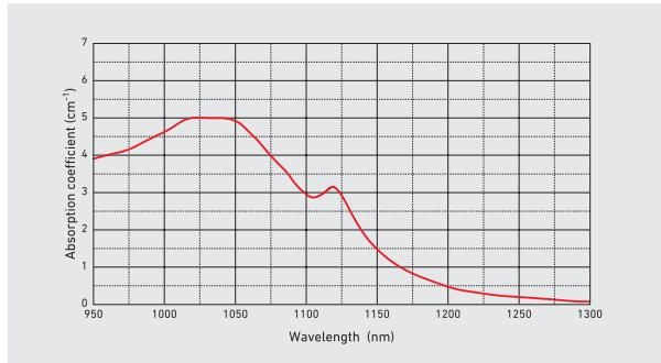
$\text{Cr}^{4+}$ :YAG crystals are ideal for passive Q-switch operation of Nd:YAG and other  $\text{Nd}^{3+}$  or  $\text{Yb}^{3+}$  doped laser crystals in the wavelength range of 900 nm to 1200 nm. Remarkable feature of  $\text{Cr}^{4+}$ :YAG is the high damage
