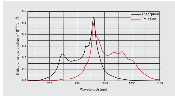
Yb<sup>3+</sup>:CaF<sub>2</sub> are among most studied and promising crystals for the development of short-pulse, high-energy, high-power diode-pumped solid-state lasers. There are several reasons that explain this trend. Firstly, calcium fluoride is a simple cubic crystal whose crystallographic properties are fairly well known.
