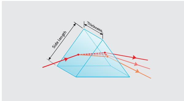
4Lasers standard uncoated isosceles dispersing prisms are fabricated from UVFS, BK7, SF11 optical glasses and offer different dispersive properties. Used in both intra- and extra-cavity setups for ultrashort
