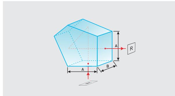
4Lasers unmounted penta prisms provide 90° beam and image deviation without inverting or reversing the image. Penta prisms reflecting surfaces are aluminized with inconel and black paint overcoat, while input and output faces are uncoated (refer to the drawing). An important feature is that these prisms do not have to be precisely
