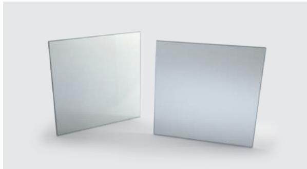
Lithium niobate (LiNbO<sub>3</sub>, LN) crystal doped with iron (Fe:LiNbO<sub>3</sub>) is an attractive photorefractive material, due to the high photorefractive sensitivity, high electro-optic coefficients and diffraction efficiency, chemo-mechanical properties. Fe:LiNbO<sub>3</sub> crystals are grown
