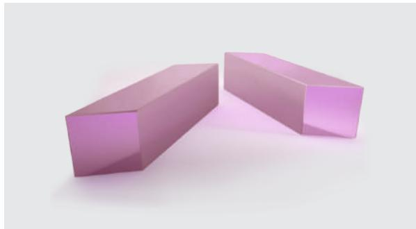
Er<sup>3+</sup>:YAG crystal is an attractive laser material for eye-safe emission at wavelengths of 1617 and 1645 nm which can be resonantly diode-pumped into the upper laser manifold at 1470 nm and 1532 nm. Due to the low quantum defect high slope efficiencies of >80% can be achieved
