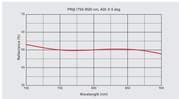
output couplers is partially reflective coated at a certain wavelength range, while the rear surface is antireflective coated in order to prevent Fresnel reflection losses. What is more, these laser cavity output couplers can be successfully implemented as fixed ratio laser power attenuators for a certain wavelength range.
