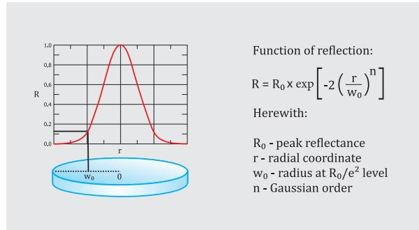
diffraction on hard-edge aperture. Therefore, super-Gaussian variable reflectivity mirrors contribute to better near- and far-field beam quality. It is worth to mention that variable reflectivity mirrors can be designed to have various reflectance profiles, such as linear, parabolic, Gaussian.
