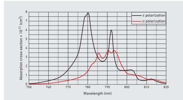
Ho<sup>3+</sup>:YAG absorption spectra and capacity of producing linearly polarized output. What is more, the refractive index of Tm<sup>3+</sup>:YLF decreases with temperature, leading to a negative thermal lens that is partly compensated by a positive lens effect due to end face bulging.
