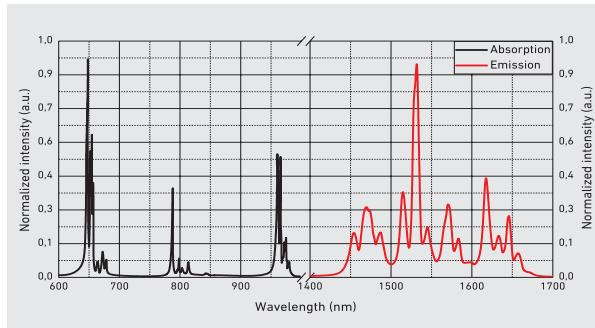
with direct fiber laser or InGaAs/InP pumping. By using heavily erbium doped (~50 at.%) YAG crystal efficient CW laser operation at ~3 μm can be obtained.
