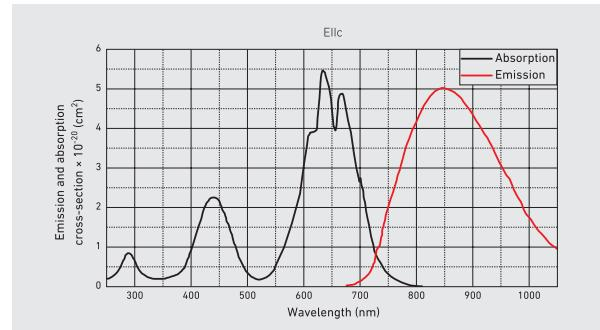
slope efficiencies above 50%. Moreover, nonlinear refractive index of Cr:LiSAF is about four times lower than that of Ti:sapphire, which reduces parasitic nonlinearities in the ultrashort pulse generation and amplification applications.
