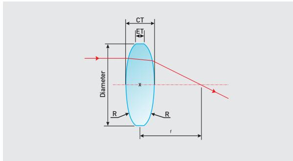
Bi-convex spherical lenses feature two convex surfaces with the same radius of curvature, while their focal length is positive. These lenses perform the best at finite conjugate (0,2X - 5X ratio) applications.
