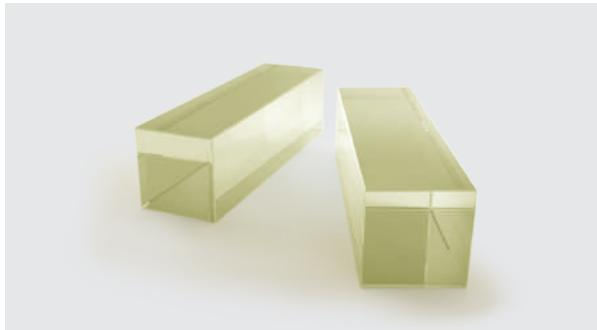
Strontium-barium niobate ( $\text{Sr}_x\text{Ba}_{(1-x)}\text{Nb}_2\text{O}_6$ , SBN:x, x = 61) crystals feature excellent optical and photorefractive properties. They are available nominally pure or doped with Ce. Different composition SBN crystals found their application in electro-optics, acousto-optics,
