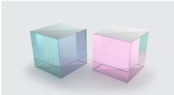
4Lasers unmounted polarizing cubes are fabricated from two identical right-angle prisms with their hypotenuse faces adhered together via optical contact or epoxy glue. Polarizing cubes are designed to transmit p-polarized light with minor deviation (<3 arcmin) and deflect s-polarized light by 90° angle. Prior to cementing polarizing dielectric thin-film coating is applied onto one of the prisms hypotenuse face, while input and exit surfaces are antireflective coated for particular
