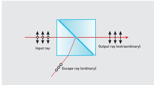
4Lasers provide air-spaced Glan-Taylor and Glan-laser type polarizers fabricated from  $\alpha$ -BBO (UV), calcite (VIS to NIR), YVO<sub>4</sub> (VIS to Mid-IR) birefringent crystalline material and mounted in a barrel-type black anodized aluminum mount. Glan-type polarizers are constructed to transmit only the extra-ordinary polarized beam, while ordinary polarized beam is deflected. These polarizers feature an extremely high extinction ratio over a wide wavelength range and their common
