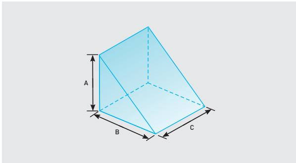
4Lasers standard uncoated right-angle ( $45^\circ$ - $90^\circ$ - $45^\circ$ ) design prisms are fabricated from UVFS and BK7 optical glasses and have three optically polished rectangular surfaces (refer to the drawing). These prisms are popular at  $90^\circ$  internal or external beam bending,  $180^\circ$  beam folding, image rotation. These applications are based on the total internal reflection at glass-air boundary inside the prism, except  $90^\circ$  external
