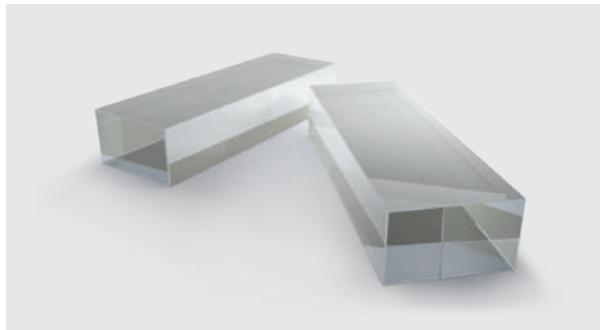
Yb<sup>3+</sup>:KYW crystals possess a large gain bandwidth that enables to obtain <100 fs pulse duration in mode-locked regime of operation. Compared with other ytterbium-doped gain media with a similarly large gain bandwidth, ytterbium-doped tungstates have fairly high emission cross-
