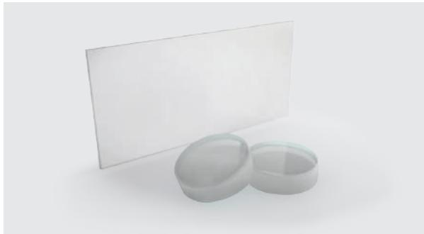
Standard uncoated flat-parallel windows are fabricated from BK7 or UV grade fused silica optical glass. UV grade fused silica glass windows are a good option for UV, ultrashort pulse, and high-power laser applications due to their low sensitivity to temperature variations, relatively high damage threshold and UV transmission down to 185 nm.
