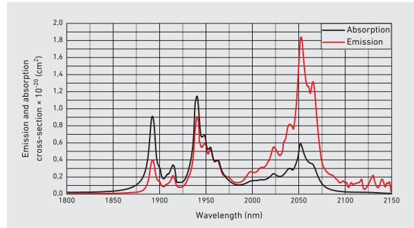
Direct pumping of Ho:YLF crystals excludes losses of Tm<sup>3+</sup> to Ho<sup>3+</sup> energy transfer process. Ho<sup>3+</sup>:YLF crystal is characterized by a long
