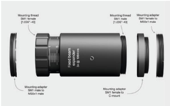
Fixed ratio beam expanders FEX series are used to increase the laser beam diameter. The FEX model diversity covers the UV, visible and NIR spectral ranges. These compact beam expanders are designed for required wavelength and have divergence adjustability.
