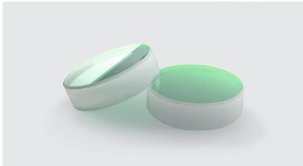
Output couplers are used in stable laser resonators in order to emit a part of the energy, which is circulating in the laser cavity. One has to carefully select the proper spatially constant reflection/transmission ratio of the output coupler in order to optimize the lasing operation and prevent from damaging intracavity optical elements. Front surface of
