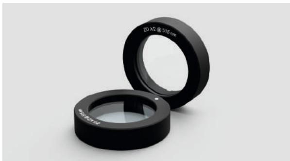
4Lasers provide mounted crystalline quartz zero-order compensated, air-spaced half-wave and quarter-wave retardance waveplates designed for a particular wavelength in the range of 257 - 1550 nm. Air-spaced construction enables these waveplates to be used for high-
