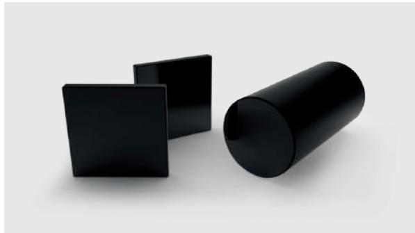
Cadmium selenide (CdSe) crystals feature an infrared transmission up to 24  $\mu\text{m}$ , reasonably large nonlinearity and small walk-off angle. CdSe crystals can be employed into difference frequency generation (DFG), optical parametric oscillation (OPO) schemes to generate infrared laser radiation above ZGP absorption edge ( $>12 \mu\text{m}$ ). For instance, CdSe OPO
