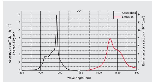
state. Fast non-radiative multi-phonon relaxation from  ${}^4\text{I}_{11/2}$  to  ${}^4\text{I}_{13/2}$  level greatly decreases the back-energy transfer and up-conversion losses due to the interaction between  $\text{Yb}^{3+}$  and  $\text{Er}^{3+}$  ions, excited at the  ${}^2\text{F}_{5/2}$  and the  ${}^4\text{I}_{11/2}$  levels, respectively.
