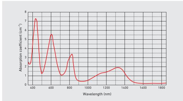
provide good lasing characteristics in passive Q-switched lasers. V:YAG features excellent optical, mechanical, and thermal properties and can be grown by Czochralski method.
