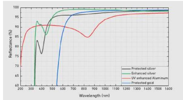
Metal-coated mirrors exhibit a relatively uniform reflectivity over wide wavelength range. They are nearly insensitive to angle of incidence and
