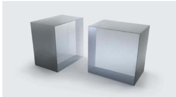
Double tungstate crystals are optically biaxial and their optical properties have to be described within the frame of optical indicatrix axes (N<sub>p</sub>, N<sub>m</sub> and N<sub>g</sub>). Advantages of Tm-doped KYW crystals include a broad fluorescence band, a large emission cross section and
