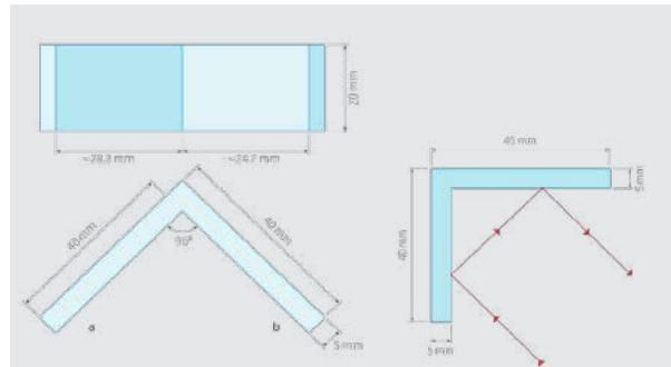
4Lasers HR right-angle retroreflectors consist of two highly reflective mirrors glued at right angle with precision as high as <30 arcsec. Hollow design eliminates the material dispersion, which is inherent in common retroreflector prisms, making them perfect for ultrashort pulse back reflection applications.
