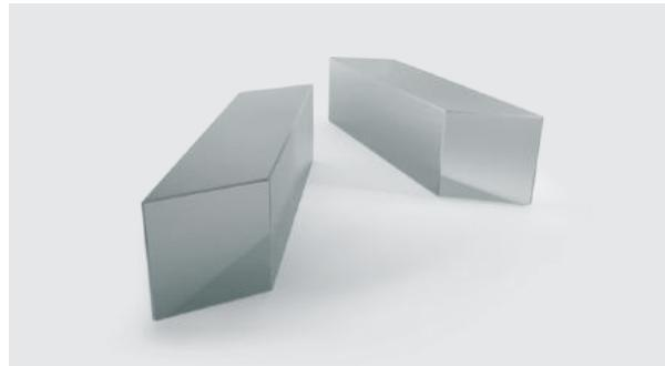
Tm<sup>3+</sup>:YLF crystal features high absorption peaks conveniently located for diode pumping around 792 nm and exhibits a cross-relaxation process, which creates two ions in the upper laser level for each pump photon absorbed. Tm<sup>3+</sup>:YLF lasers are ideal pump sources for Ho<sup>3+</sup>:YAG lasers. This is due to a good overlap of Tm<sup>3+</sup>:YLF emission and
