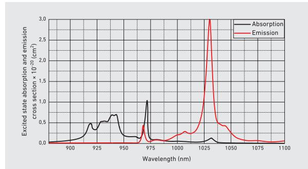
Yb<sup>3+</sup>:YAG crystals feature a 950 μs lifetime of the  ${}^2F_{5/2}$  ytterbium energy level and a quantum defect of only ~9%. Yb:YAG crystals also possess a broad pump band at near 940 nm that is more than 10 times broader than the 808 nm pump line of Nd:YAG crystals. It makes Yb:YAG systems
