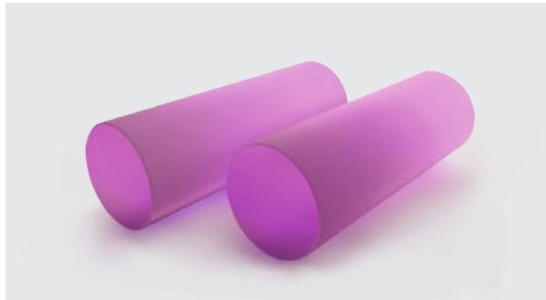
Nd<sup>3+</sup>:YAG crystal is the most widely used solid-state laser material. These crystals are characterized by relatively small gain bandwidth, which allows achieving a high gain efficiency and a relatively low lasing threshold.
