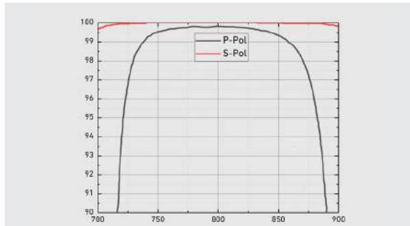
Low GDD Ultrafast mirrors are designed for high power ultrashort (femtosecond) laser pulse applications to provide both maximized high reflectivity and minimized low GDD value at the same time. Such coatings are used for internal and external beam manipulation applications where pulse broadening effect is undesirable.
