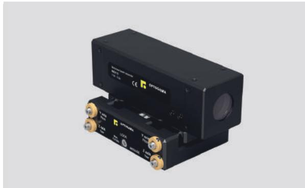
Motorized laser beam expanders MEX series are used to increase the laser beam diameter and adjust divergence. Standard or custom-made beam expanders feature a unique mechanical closed loop sliding-lens design ensuring high pointing stability and minimal dimensions.
