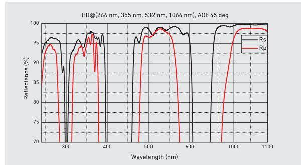
Dual and multi wavelength mirrors provide a high reflectance over several certain spectral ranges at a specific angle of incidence and polarization for non-normal incidence. Reflectance properties are based
