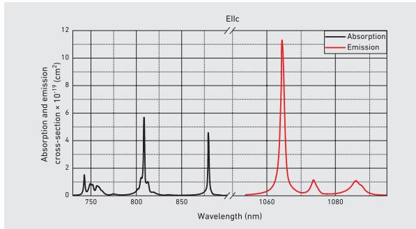
impossible to achieve pulse energies as high as it is achievable with Nd:YAG lasers at Q-switched operation, due to the lower upper-state lifetime and higher gain efficiency. In conclusion, Nd:YVO<sub>4</sub> is better suited as an active medium of high pulse repetition rate Q-switched lasers and CW lasers with a lower lasing threshold.
