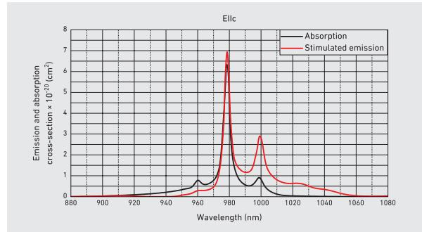
and absorption cross-sections are strongly dependent upon the crystallographic orientation. The absorption cross-sections of the Yb:YAP crystal is higher than that of the Yb:YAG crystal.
