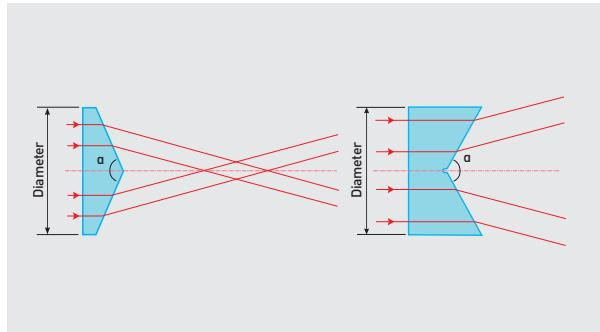
Axicons (conical lenses) are famous for their ability to transform a collimated Gaussian beam into an approximation of non-diffracting Bessel beam in the near-field and ring-shaped beam in the far-field. Most often they are used in tandem with other types of lenses. 4Lasers
