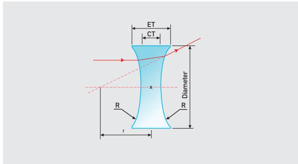
Bi-concave spherical lenses feature two spherical concave surfaces with the same radius of curvature, while their focal length is negative. The performance of these lenses is best when used for finite
