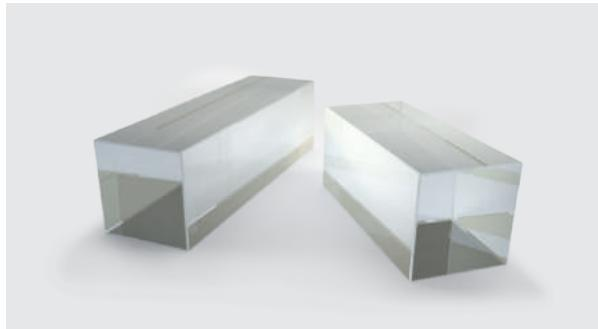
$\text{Er}^{3+},\text{Yb}^{3+}$  co-doped phosphate glass (Er,Yb:phosphate glass) is a well-known and commonly used active medium for lasers emitting in the "eye-safe" spectral range of 1.5-1.6  $\mu\text{m}$ . Phosphate glass combines a long lifetime ( $\sim 8$  ms) of  ${}^4\text{I}_{13/2}\text{Er}^{3+}$  upper laser level with a low (2-3 ms) lifetime of  ${}^4\text{I}_{11/2}\text{Er}^{3+}$  level that is in resonance with  $\text{Yb}^{3+} {}^2\text{F}_{5/2}$  excited
