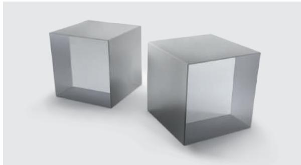
Compared to Nd<sup>3+</sup>:YAG crystals, the Nd<sup>3+</sup>:YVO<sub>4</sub> crystal has much higher absorption and emission cross-sections, a broader gain bandwidth and wavelength range for pumping, a shorter upper-state lifetime, a higher refractive index, thus it is characterized by a lower thermal conductivity. Nd:YVO<sub>4</sub> crystals are well suited for passively mode-locked lasers with high pulse repetition rates. A drawback of Nd:YVO<sub>4</sub> lasers is that it is
