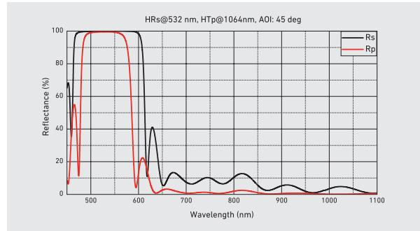
Wavelength separators and combiners provide spatial separation or combination of different spectral components. These optical elements feature highly reflective dielectric coatings on the front side and
