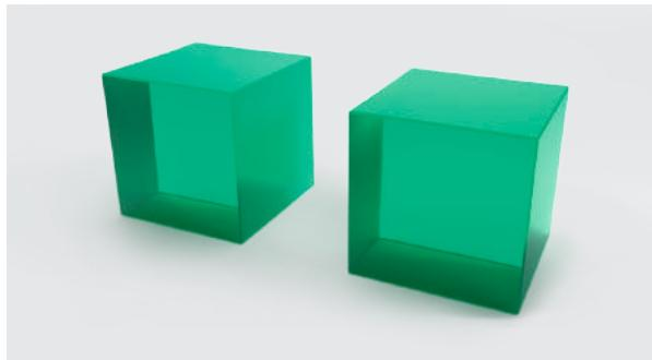
$\text{Cr}^{3+}$ :LiSAF gain medium possesses a broad emission band in the near infrared that allows a widely tunable laser operation and generation of  $\sim 10$  fs light pulses via mode-locking technique. Cr:LiSAF crystals can be grown with a very low loss level ( $<0.2\%/\text{cm}$ ). It enables to construct high-Q-cavities, resulting in lasing thresholds as low as 2 mW and
