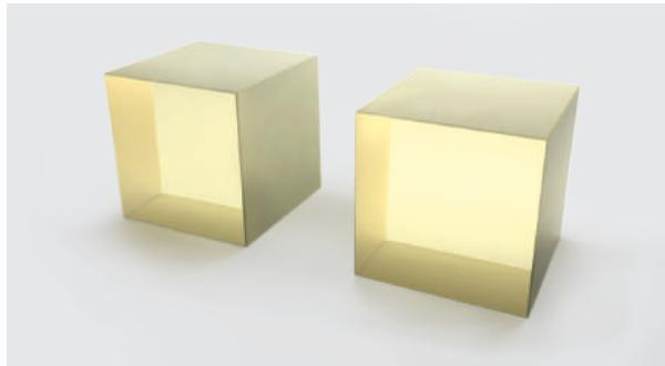
Very few laser materials have necessary properties for realization of lasing in the visible spectral range. Trivalent praseodymium ( $\text{Pr}^{3+}$ ) is known to be an interesting laser ion for using with solid-state lasers in the visible spectral range because of its energy levels scheme, providing several transitions in the red (640 nm,  ${}^3\text{P}_0$  to  ${}^3\text{F}_2$ ), orange (607 nm,  ${}^3\text{P}_0$
