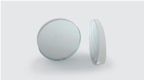
Windows with a slight wedge are commonly used to prevent harmful laser cavity feedback and beam interference effects. Standard 4Lasers uncoated flat-wedge windows are fabricated from BK7 and UV grade fused silica optical glass. UV grade fused silica glass flat-wedge window is a good option for UV, ultrashort pulse and high-power laser
