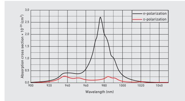
transfer (~94%) and weak up conversion losses due to the very short lifetime of  ${}^4\text{I}_{11/2}$  excited state (~80 ns) facilitated by a high maximum phonon energy of the host material ( $\hbar\nu_{\max} \sim 1500 \text{ cm}^{-1}$ ). A strong and wide (~17 nm) absorption band is observed at 976 nm that coincides with the emission spectrum of InGaAs laser diodes.
