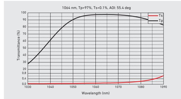
for high-power and UV applications. 4Lasers design and manufacture standard and custom Brewster type polarizers in the range of 230 nm and 2000 nm with face dimensions up to 160 mm.
