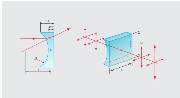
Plano-concave cylindrical lenses feature single plano, single concave cylindrical surface and negative focal length. These lenses are similar to plano-concave spherical lenses, though the difference is that they
