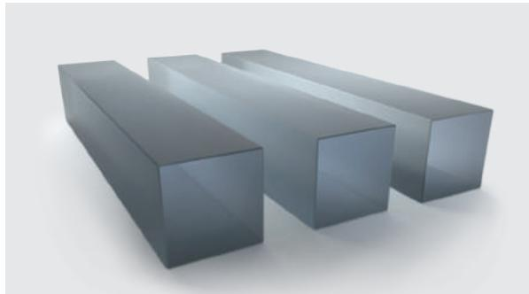
Potassium yttrium tungstate ( $\text{KY(WO}_4)_2$ , KYW) crystals offer two strong phonon modes around  $765 \text{ cm}^{-1}$  and  $905 \text{ cm}^{-1}$ , which have similar Raman gain and are pump polarization dependent. KYW crystals
