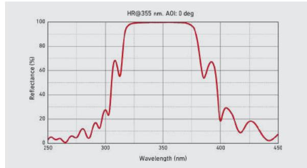
Laser line mirrors exhibit high reflectance over a particular spectral range, extending <10% of the central wavelength, at a specific angle of incidence and polarization for non-normal incidence. Reflectance
