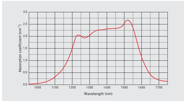
Co:Spinel is a recently developed material, which has been proven to be a very effective passive Q-switch in lasers emitting in the range of 1.2  $\mu\text{m}$  - 1.6  $\mu\text{m}$ . Co:Spinel has a high absorption cross-section, which permits Q-switch operation of Er:glass laser (both flash-lamp and diode-
