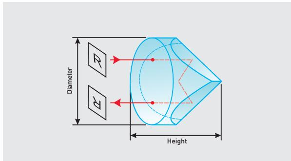
4Lasers standard uncoated corner cube retroreflectors are fabricated from high-quality UVFS and BK7 optical glasses. Corner cube retroreflector prisms provide the beam deviation by  $180^\circ$  and creates an inverted, reversed image independent of the angle of incidence, with a wide incident angle acceptance range. Operating principle is based on
