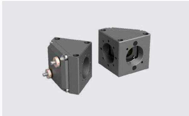
XY-IND are 2-axis and 3-axis sealed industrial kinematic mirror/splitter mounts. It combines with sealing tubes in both ends for optics and laser beam path protection from dust and environment. The mounts are easily attached together at any direction.
