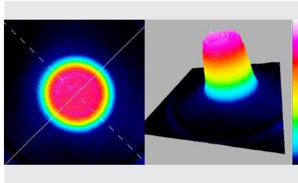
Flat top converter unit is "all in one" motorized solution for a Gaussian beam transformation to a Flat-Top (Top Hat) beam. The beam profile remains Flat-Top shape along optical axis. The device consists of quartz wave-plate, space-variant wave-plate and a high contrast polarizer. The FTC is produced in the UV, visible and NIR spectral ranges, from 250 nm to 2000 nm.
