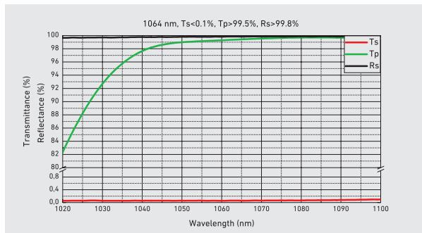
wavelength range. 4Lasers optically contacted polarizing cubes provide higher laser induced damage threshold, therefore are primarily used for high-power applications, while epoxy glued cubes are a cost-effective choice for low and mid-power applications. We recommend to use these elements with collimated laser beams in order to avoid beam aberrations.
