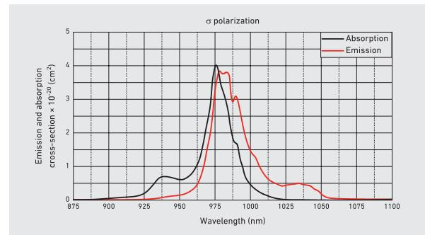
High concentrations of Yb<sup>3+</sup> ions can be included in the YAB crystal matrix with little concentration quenching. Yb:YAB crystals feature good mechanical strength, good thermal conductivity, and stable chemical characteristics.
