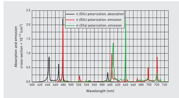
to  ${}^3\text{H}_6$ ), green (532 nm,  ${}^3\text{P}_0$  to  ${}^3\text{H}_5$ ), and dark red (720 nm,  ${}^3\text{P}_0$ ,  ${}^3\text{F}_3 + {}^3\text{F}_4$ ) spectral regions.  $\text{Pr}^{3+}\text{:YLF}$  has been found to be a promising laser material for producing visible lasers directly and UV lasers through intracavity second-harmonic generation.
