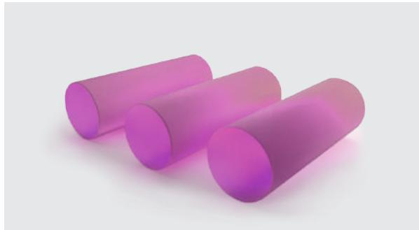
Nd<sup>3+</sup>:YLF crystal is characterized by a long lifetime of  ${}^4F_{3/2}$  neodymium energy level. Compared to Nd:YAG, the lower thermal conductivity and a weak negative dn/dT lead to lower thermal distortions and allow
