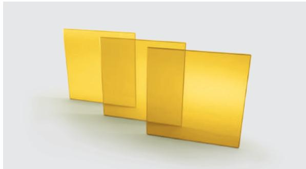
Bismuth silicone oxide ( $\text{Bi}_{12}\text{SiO}_{20}$ , BSO) crystals are highly efficient photoconductors with a low dark conductivity, that allows a build-up of large photo-induced space-charges. Tremendous photoconductivity and electro-optic properties make BSO crystals attractive in a range
