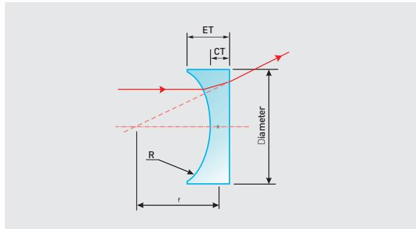
Plano-concave spherical lenses have one plano and one spherical concave surface, while their focal lengths are negative. These lenses provide the best performance when used for 5X to infinite-conjugate
