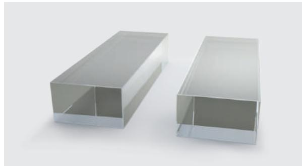
$\text{Yb}^{3+}$ :KGW crystals possess a large gain bandwidth that enables to obtain <100 fs pulse duration in mode-locked regime of operation. Compared with other ytterbium-doped gain media with a similarly large gain bandwidth, ytterbium-doped tungstate has fairly high emission cross-sections. Ytterbium doping concentration in Yb:KGW crystals can
