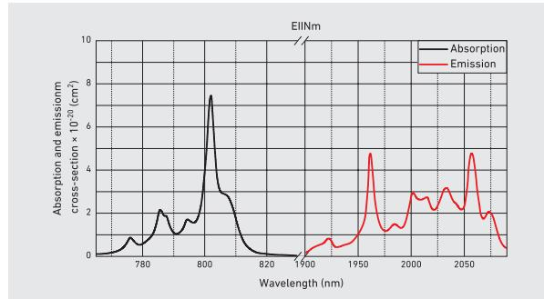
therefore co-doping of  $\text{Ho}^{3+}$  with  $\text{Tm}^{3+}$  is chosen for an efficient operation across the 2  $\mu\text{m}$  region through the energy transfer route from  $\text{Tm}^{3+}$  to  $\text{Ho}^{3+}$ . Tm, Ho:KYW crystals are characterized by large and broad polarized absorption and emission bands, efficient energy transfer from  $\text{Tm}^{3+}$  to  $\text{Ho}^{3+}$ .
