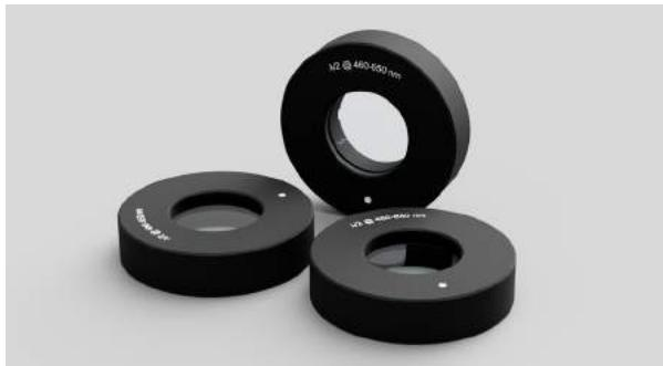
4Lasers provide mounted achromatic (broadband) half-wave and quarter-wave retardance waveplates for several bands in the wavelength range of 460 nm - 1700 nm. Air-spaced construction enables to use these waveplates for high-power applications. These
