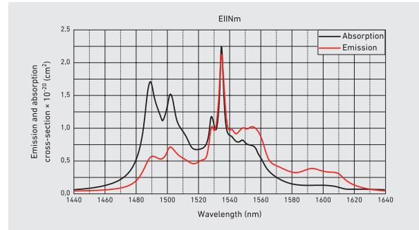
Er<sup>3+</sup>:KYW is a promising laser material for eye-safe emission at the wavelength of 1609 nm, which can be resonantly diode-pumped into the upper laser manifold at 1534 nm. Due to the low quantum defect high-slope efficiencies of >80% can be achieved with direct fiber laser
