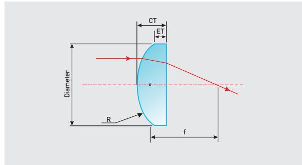
Plano-convex spherical lenses have one plano and one spherical convex surface, while their focal lengths are positive. These lenses provide the best performance when used for 5X to infinite-conjugate ratio
