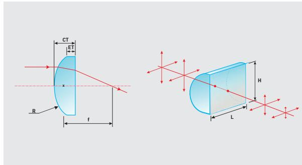
Plano-convex cylindrical lenses feature single plano and single convex cylindrical surface, while their focal length is positive. These lenses operate only in one dimension rather than two, compared to plano-
