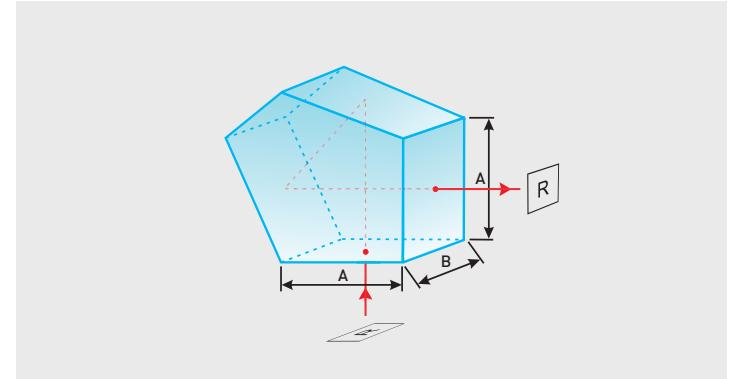
4Lasers unmounted penta prisms provide 90° beam and image deviation without inverting or reversing the image. Penta prisms reflecting surfaces are aluminized with inconel and black paint overcoat, while input and output faces are uncoated (refer to the drawing). An important feature is that these prisms do not have to be precisely aligned to operate properly. Therefore,
