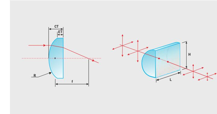
Plano-convex cylindrical lenses feature single plano and single convex cylindrical surface, while their focal length is positive. These lenses operate only in one dimension rather than two, compared to plano-convex spherical
