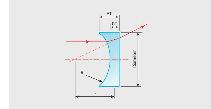
collimating a convergent beam, diverging a collimated beam. To prevent spherical aberrations collimated beam should always be incident on curved lens surface and vice versa.
