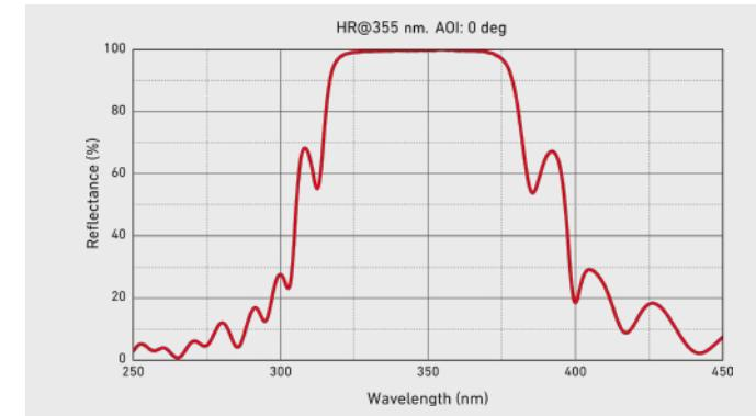
on the optical interference phenomena of reflections from multiple dielectric thin-film layers, which are carefully deposited on UV grade fused silica optical substrates.
