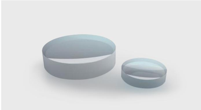
Plano-concave spherical lenses have one plano and one spherical concave surface, while their focal lengths are negative. These lenses provide the best performance when used for 5X to infinite-conjugate ratio applications, e.g.
