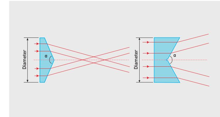
Axicons (conical lenses) are famous due to their ability to transform a collimated Gaussian beam into an approximation of non-diffracting Bessel beam in the near-field and ring-shaped beam in the far-field. Most often they are used in tandem with other types of lenses. 4Lasers provide plano-convex
