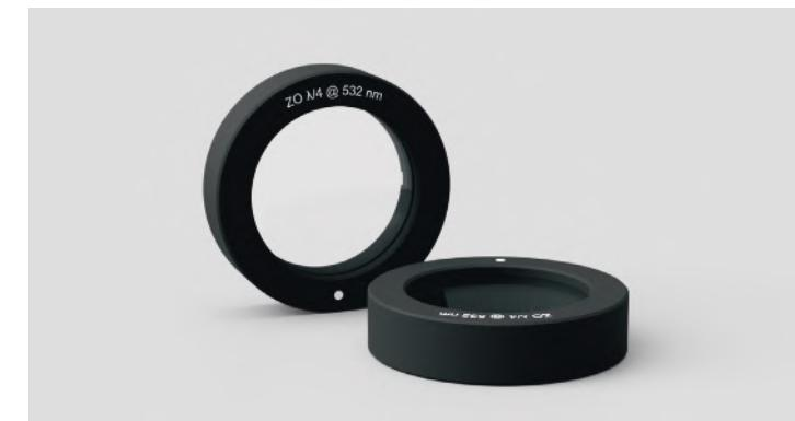
Air-spaced construction enables these waveplates to be used for high-power applications, while zero-order design features lower temperature and wavelength dependence compared to low and multiple order waveplates.
