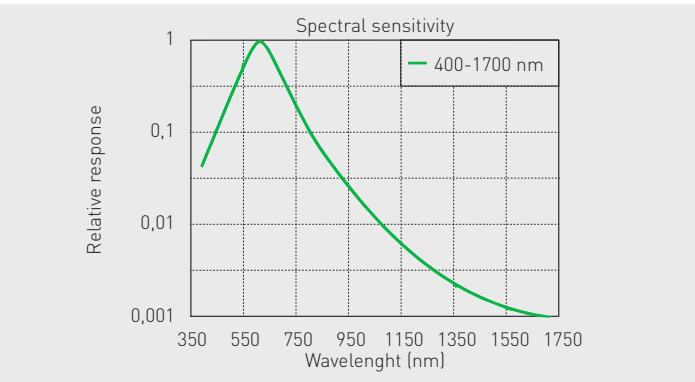
The near infrared Contour-IR camera is designed for observation, registration and recording radiation in the near infrared zone of the 400 - 1700 nm spectral region emitted by infrared sources such as GaAs IR LED, diode or solid-state lasers as well as for use in infrared microscopy, infrared luminescence, examination of documents, forensics, art restoration and etc.
