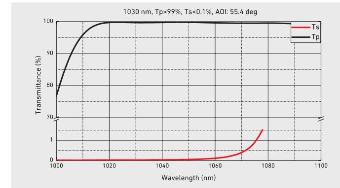
4Lasers standard high contrast Brewster-type and 45° thin-film polarizers provide high extinction ratio Tp:Ts > 1000:1 thanks to the ion beam sputtered (IBS) thin-film coatings. Moreover, these polarizers are ideal for high-power levels and UV wavelength range. 4Lasers design and manufacture standard
