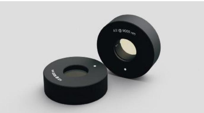
4Lasers provide unique zero-order, monolithic design mid-infrared (MWIR and LWIR) waveplates mounted in  $\varnothing 25.4 \times 6$  mm black anodized metal mount for the range of 3500 nm - 10600 nm. These waveplates are available with quarter-wave, half-wave or any other custom retardance. Each MWIR
