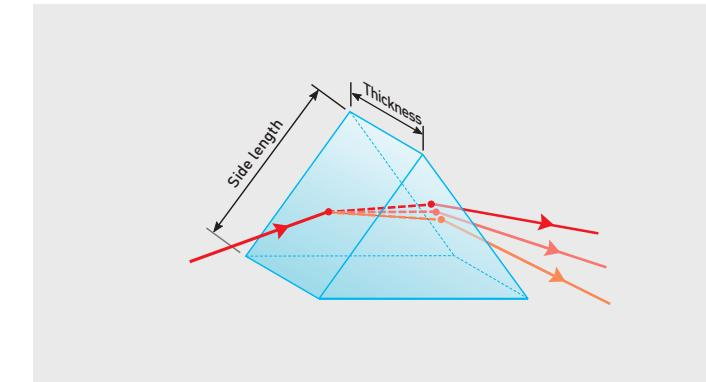
4Lasers standard uncoated isosceles dispersing prisms are fabricated from UVFS, BK7, SF11 optical glasses and offer different dispersive properties. Used in both intra- and extra-cavity setups for ultrashort laser pulse temporal
