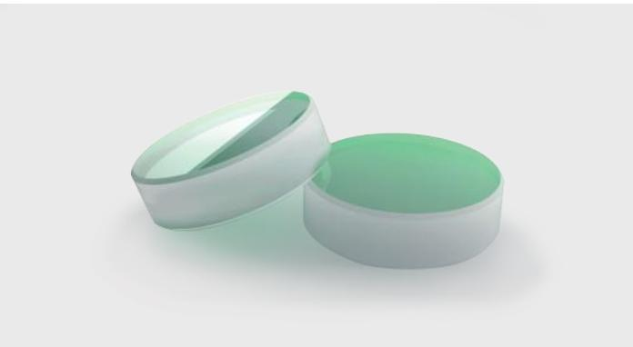
Output couplers are used in stable laser resonators in order to emit a part of the energy, which is circulating in the laser cavity. One has to carefully select the proper spatially constant reflection/transmission ratio of the output coupler in order to optimize the lasing operation and prevent from damaging intracavity optical elements. Front surface of output couplers is partially
