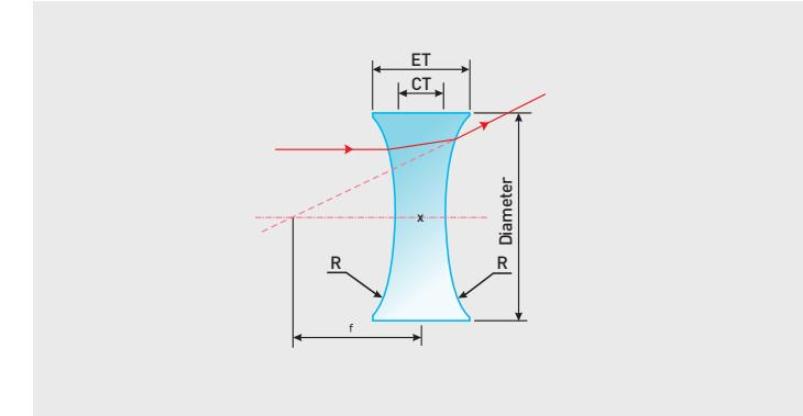
Bi-concave spherical lenses feature two spherical concave surfaces with the same radius of curvature, while their focal length is negative.
