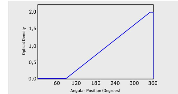
By using two filters in combination in reverse rotation can obtain a fixed density attenuation and extends the number applications. Sizes are available from 25 mm to 100 mm in diameter.
