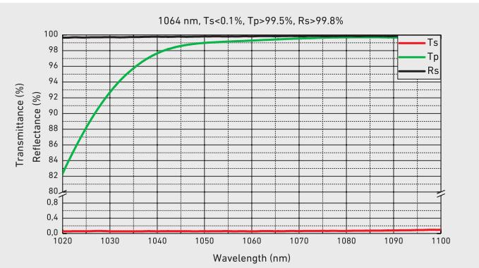
antireflective coated for particular wavelength range. 4Lasers optically contacted polarizing cubes provide higher laser induced damage threshold, therefore are primarily used for high-power applications, while epoxy glued cubes are a cost-effective choice for low and mid-power applications. We recommend to use these elements with collimated laser beams in order to avoid beam aberrations.
