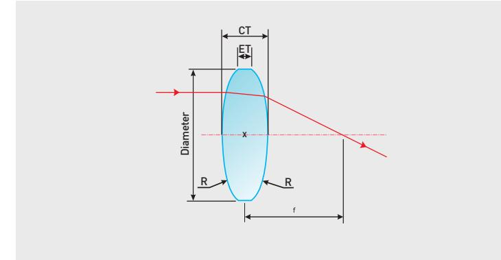
Bi-convex spherical lenses feature two convex surfaces with the same radius of curvature, while their focal length is positive. These lenses perform the
