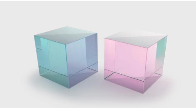
4Lasers unmounted polarizing cubes are fabricated from two identical right-angle prisms with their hypotenuse faces adhered together via optical contact or epoxy glue. Polarized cubes are designed to transmit p-polarized light with minor deviation (<3 arcmin) and deflect s-polarized light by 90° angle. Prior to cementing polarizing dielectric thin-film coating is applied onto one of the prisms hypotenuse face, while input and exit surfaces are
