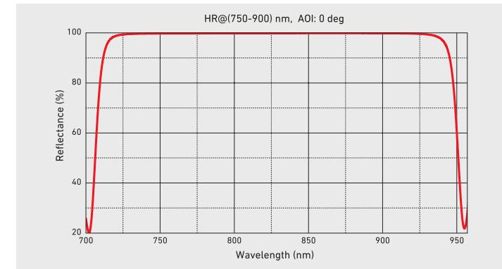
Broadband laser mirrors provide high average reflectance over a broad spectral range at a specific angle of incidence and polarization for non-normal incidence. These properties are based on the optical interference
