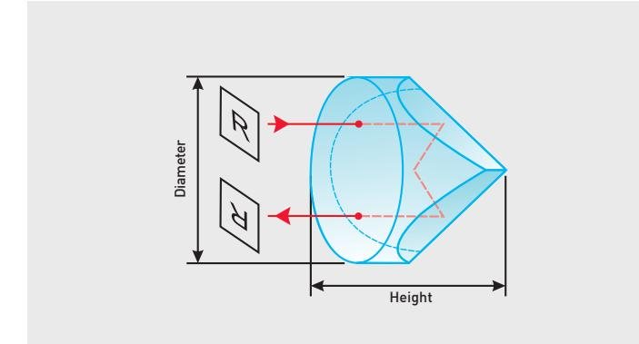
4Lasers standard uncoated corner cube retroreflectors are fabricated from high-quality UVFS and BK7 optical glasses. Corner cube retroreflector prisms provide the beam deviation by 180° and creates an inverted, reversed image independent of the angle of incidence, with a wide incident angle acceptance
