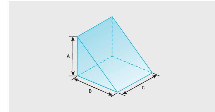
4Lasers standard uncoated right-angle ( $45^\circ$ - $90^\circ$ - $45^\circ$ ) design prisms are fabricated from UVFS and BK7 optical glasses and have three optically polished rectangular surfaces (refer to the drawing). These prisms are popular at  $90^\circ$  internal or external beam bending,  $180^\circ$  beam folding, image rotation. These applications are based on the total internal reflection at glass-
