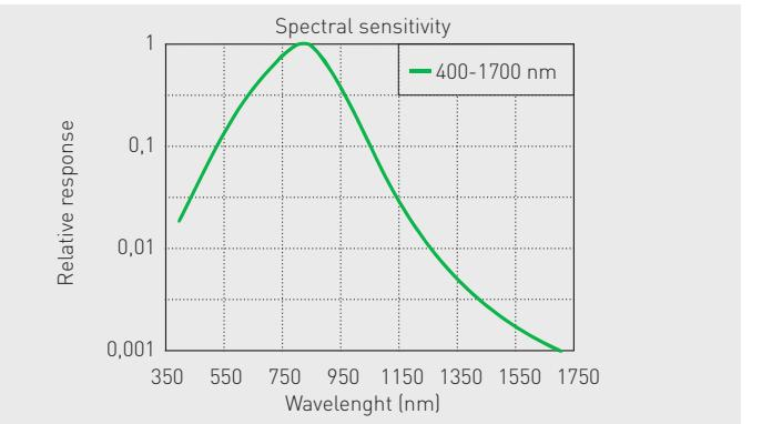
The near infrared Contour IR Digital camera is designed for observation, registration and recording radiation in the near infrared zone of the 400 - 1700 nm spectral region emitted by infrared sources such as GaAs IR LED, diode or solid-state lasers as well as for use in infrared microscopy, infrared luminescence, examination of documents, forensics, art restoration, etc.
