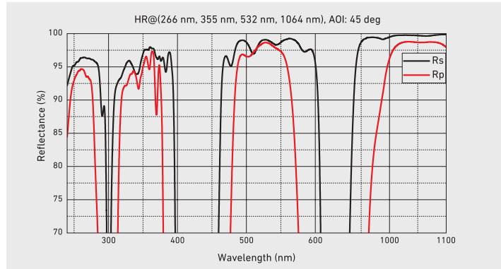
Dual ant multi wavelength mirrors provide a high reflectance over several certain spectral ranges at a specific angle of incidence and polarization for non-normal incidence. Reflectance properties are based on the optical
