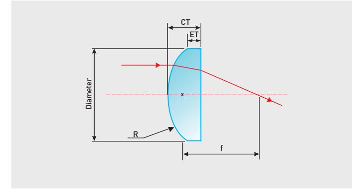
performance when used for 5X to infinite-conjugate ratio applications, e.g. focusing a collimated light beam or collimating beam from a point source.
