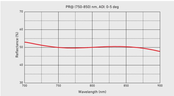
reflective coated at a certain wavelength range, while the rear surface is antireflective coated in order to prevent Fresnel reflection losses. What is more, these laser cavity output couplers can be successfully implemented as fixed ratio laser power attenuators for a certain wavelength range.
