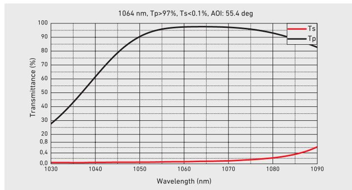
4Lasers standard Brewster-type thin-film polarizers are designed for applications, which include polarization separation. These elements provide a moderately extinction ratio  $T_p:T_s > 200:1$  and are perfectly fit for high-power
