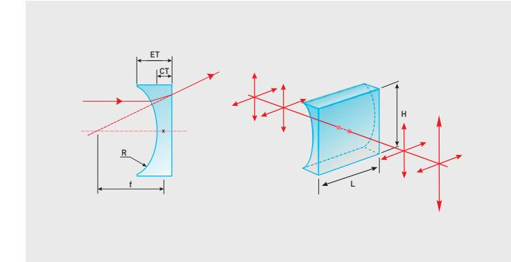
only in a single dimension rather than two symmetrical dimensions. Applicable conditions for optimal performance are the same as for plano-concave lenses: from 5X to infinite-conjugate ratio.
