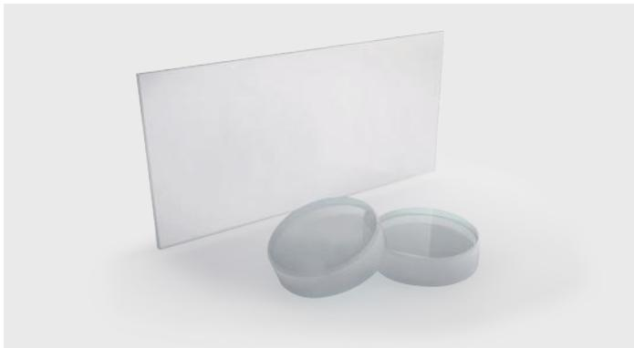
Standard uncoated flat-parallel windows are fabricated from BK7 or UV grade fused silica optical glass. UV grade fused silica glass windows are a good choice for visible and near-infrared range, low/mid-power laser and non-laser applications. These components are initially uncoated and demand metallic or dielectric coatings for a particular application. 4Lasers provide coating service upon request. Contact us for custom solutions and pricing.
